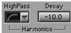
**Highpass filter toggle** - removes low frequencies from the generated harmonics. First position is a 24dB/oct filter at 16Hz (basically to remove DC and very low frequency components); second position is a 12dB/oct filter at the selected Frequency on the graph; third position is a 24dB/oct filter at the selected Frequency on the graph. Default is 12dB/oct.
