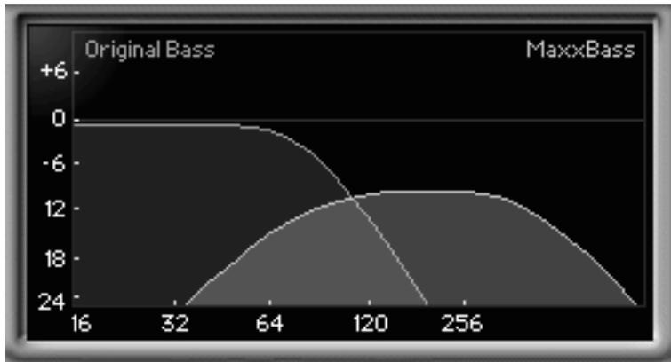
Recommended settings to start with for mixing and mastering are the defaults. Simply increase the Harmonic fader to add to the mix (shown by the yellow curve in the graphic). The best Frequency will be usually between 60 and 100. Your goal should be a smooth, warm bass response that is balanced, not more bass than you usually would use.
