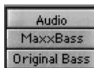
**Monitor button** - selects between Audio (the normal mixed output), Harmonics (the signal created by MaxxBass), and Original Bass.
