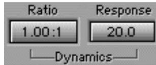
Ratio and Response controls let you alter the dynamic nature of the harmonics. There is a compressor in the MaxxBass processor that affects only the harmonics, not the Original Bass.
