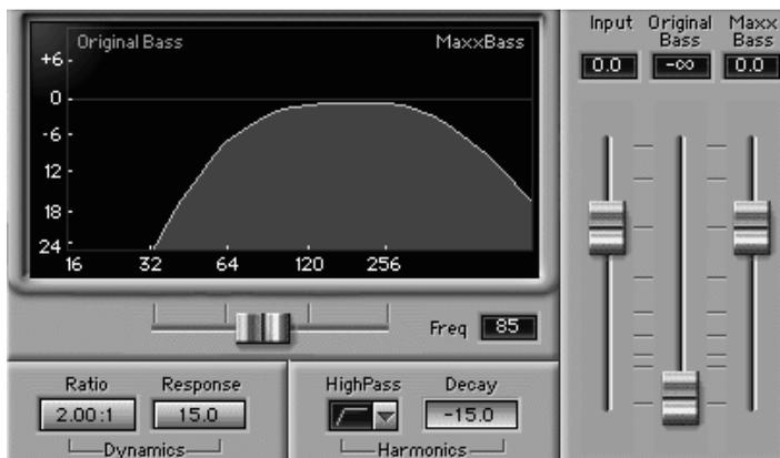
With these settings you should find that the bass response is improved by using the MaxxBass signal instead of the Original Bass, and that you can get an overall louder level (this is due to the fact that the little speakers are not challenged so much by the low frequencies they can not reproduce well).
