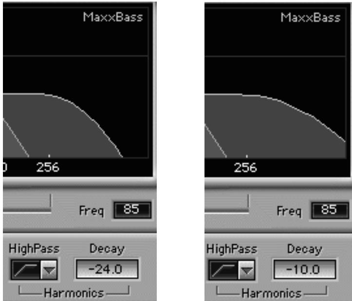
The Decay control is subtle, but important, and rather source-dependant. With higher values (closer to zero), the number of harmonics and their levels is increased. If you have a high-input signal, and high Decay values, you may have internal clipping. Reduce the Input control to allow more internal headroom.
