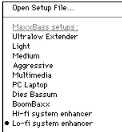
Listed here are the factory presets of MaxxBass, which are intended only as starting points, not actual solutions. You must adjust each setup for the source material.
