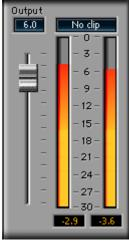
This control sets the overall output gain. It can be used to prevent output clipping.
